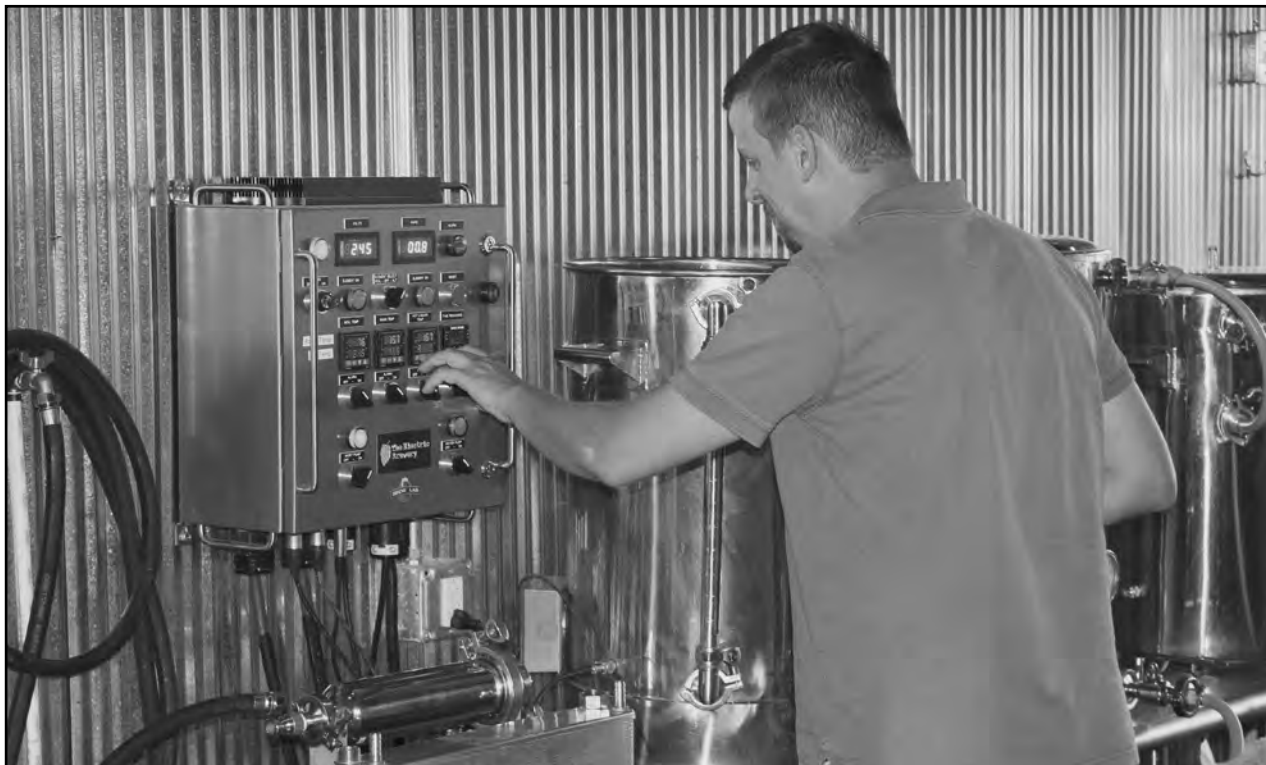
DIALING IN: Wichitan David Bosarge adjusts the timer on the electric brewing control system at Brew Lab in Overland Park.
